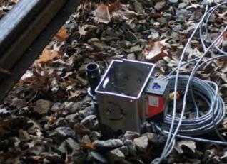
In this test, we proved the effectiveness of Dimetix laser distance sensors coupled with interface modules produced by Laser-View Technologies as a crucial tool to acquire deflection accurately in real-time. The laser system provided methods that will be beneficial across many bridge testing practices.
