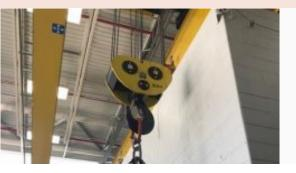
In low overhead situations, the hoist can interfere with structures or equipment on the factory floor under the crane runway. Other situations exist in which a die may need to be transported through the facility and needs a clear path so that collisions will not occur. No-fly zone systems add to a company's safety program.
